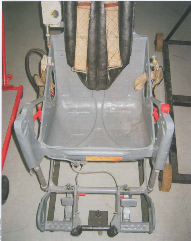
Pilot's seat with visible cavity which housed parachute • Miska spadochronowa fotela z podnóżkami
