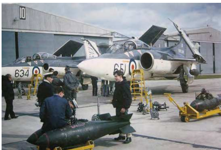
▲ A Buccaneer S.2 (right) and an S.1 – note the engine air intake sizes – of 736 NAS being loaded with live 1,000lb bombs at Brawdy, Wales, before a further sortie against Torrey Canyon
