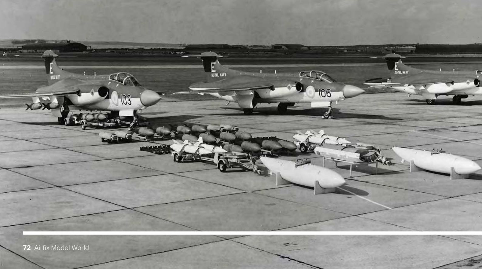
Buccaneers of 800 NAS at Lossiemouth with an extensive display of weapons. These include underwing fuel tanks, AGM-12 Bullpup missiles, 1,000lb bombs, Gloworm flare rockets and 2in rocket pods
