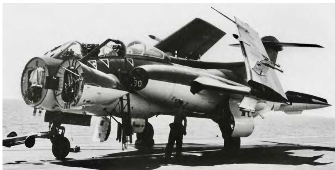
▲ With everything folded, XN959 is ready to be lowered to the hangar on the for'ard lift. It is fitted with a twin-store practice bomb carrier on the inboard pylon, while a Gloworm flare rocket rail unit is fixed to the outboard pylon
