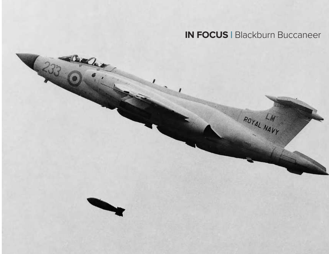
▲ A primary mode for the delivery of 1,000lb bombs – and a nuclear store – was a toss manoeuvre. This all-white S.1, XN965 of 700 Z Flight, tosses a thousand-pounder from its large rotary bomb bay
